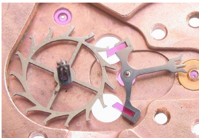
Calibre 551 escape wheel and pallet lever showing the jewelled entry and exit pallets
