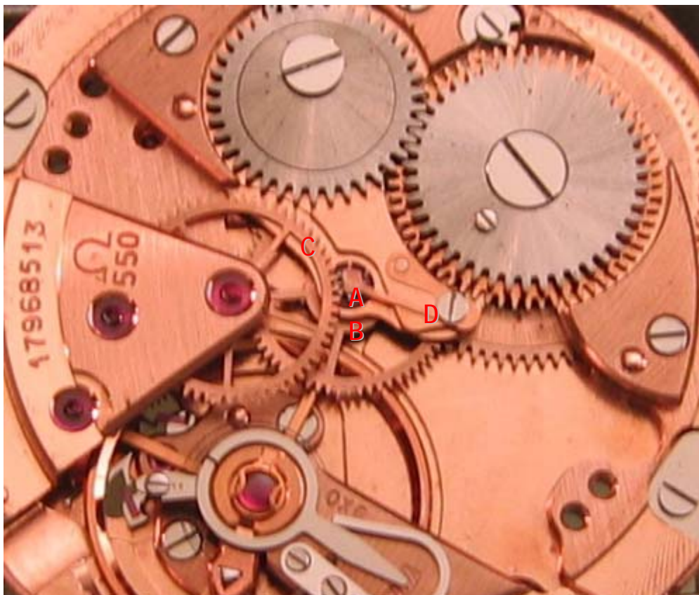
The sweep seconds pinion A (just visible) passes through the centre wheel B. The third wheel C drives the pinion A. Resting on the pinion A is the sweep seconds friction spring D that stabilises the sweep second hand motion preventing the jerky action that can occur owing to play between the teeth of the third wheel and those of the sweep second pinion. Notice the visibility and access of the balance wheel. Photo: courtesy Jim Hodek
