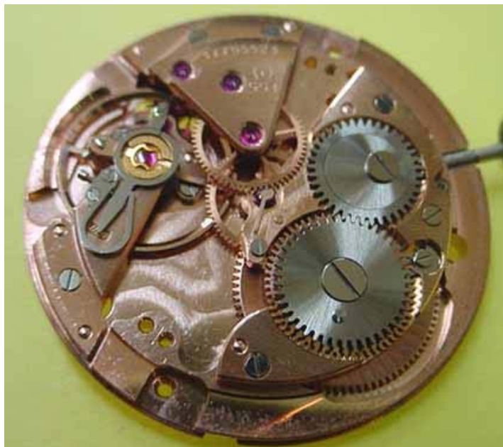
Snailing on crown and ratchet wheels. Notice damascening of the plate, producing a play of light that looks similar to mother of pearl
