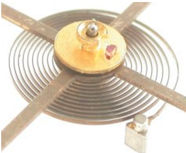
Calibre 551 Nivarox balance spring made from an iron, nickel, beryllium, titanium and silicon alloy. Notice the highly polished tempered alloy pivot.
